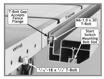
Figure 8. Front rail being slid onto T-bolts.
